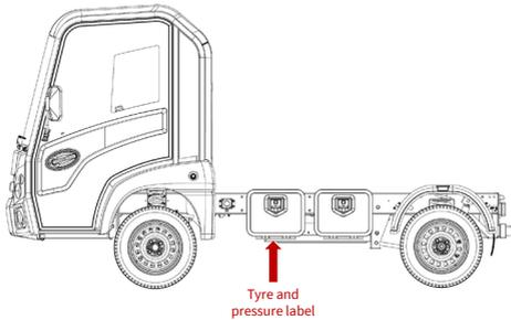
Figure 19 - Tyre and pressure label
