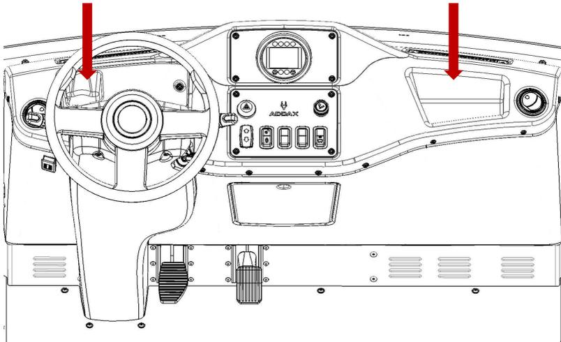
Figure 17 - Front storage compartment combined with cup holder
