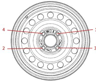
Figure 26 - Wheel nut position
