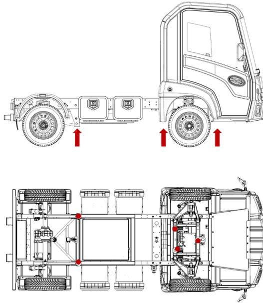
Figure 25 – Front and rear jacking points
