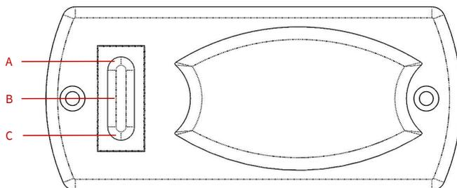
Figure 13 - Interior light switch
