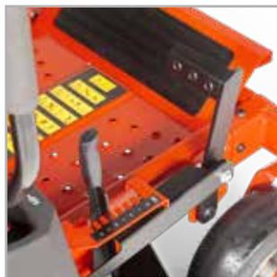
**FOOT-ASSISTED MOWER DECK LIFT**
